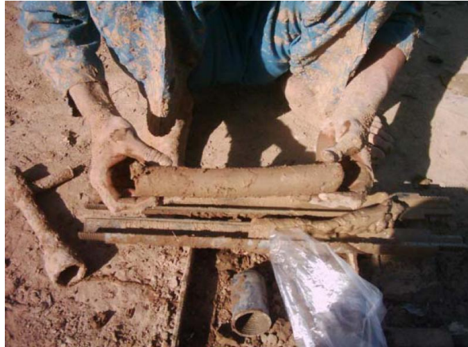
Site Photo 21. Split spoon sample (Courtesy of USACE)
