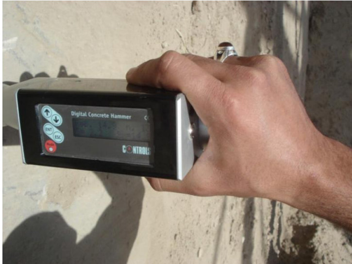
Site Photo 14. Hammer test for elevated storage tank (Courtesy of the USACE)
