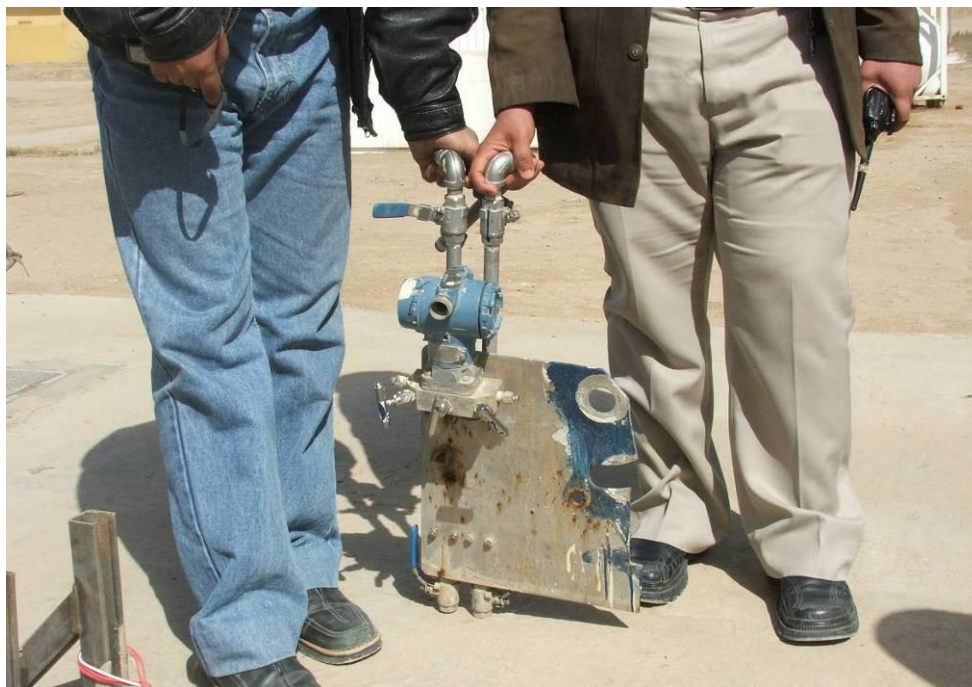
Site Photo 11. The disabled flow meter for the HSPS meter vault
