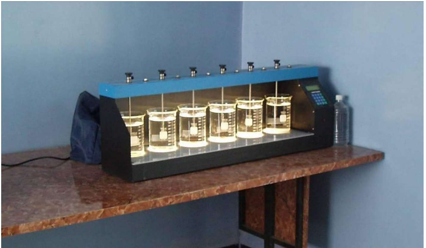
Site Photo 27. Nassriya WTP laboratory equipment required to perform jar tests (Photo courtesy of ITAO)
