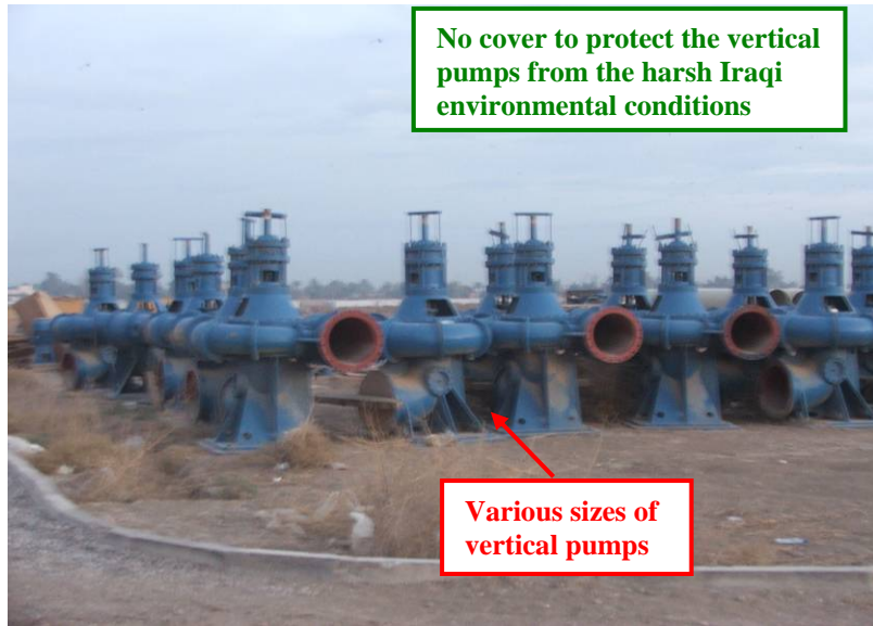
Site Photos 36 and 37. Vertical pumps, motors, and accessories located behind the GRC HQs living quarters
