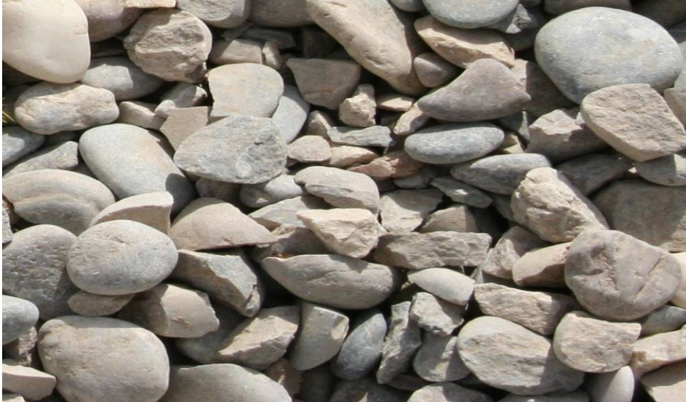
Site Photo 5. Crush aggregate used in concrete mix for tank foundation.
