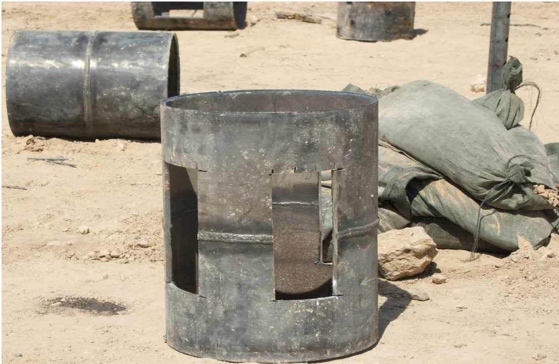
Site Photo 12: Test Section Cut for Destructive Test
