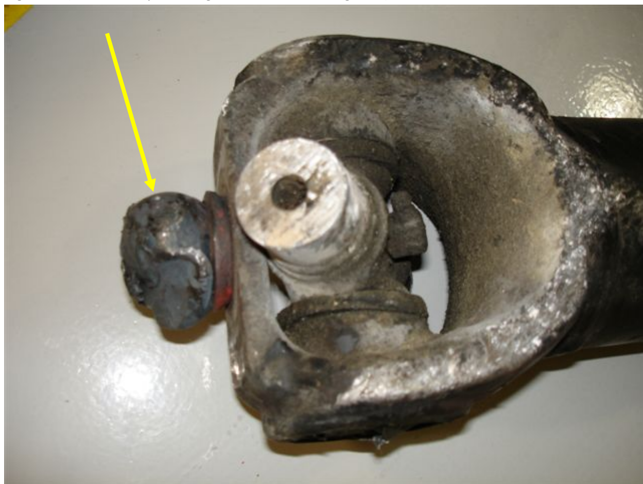
Figure 2a (Note close up of bluing of ball due to lack of grease)
