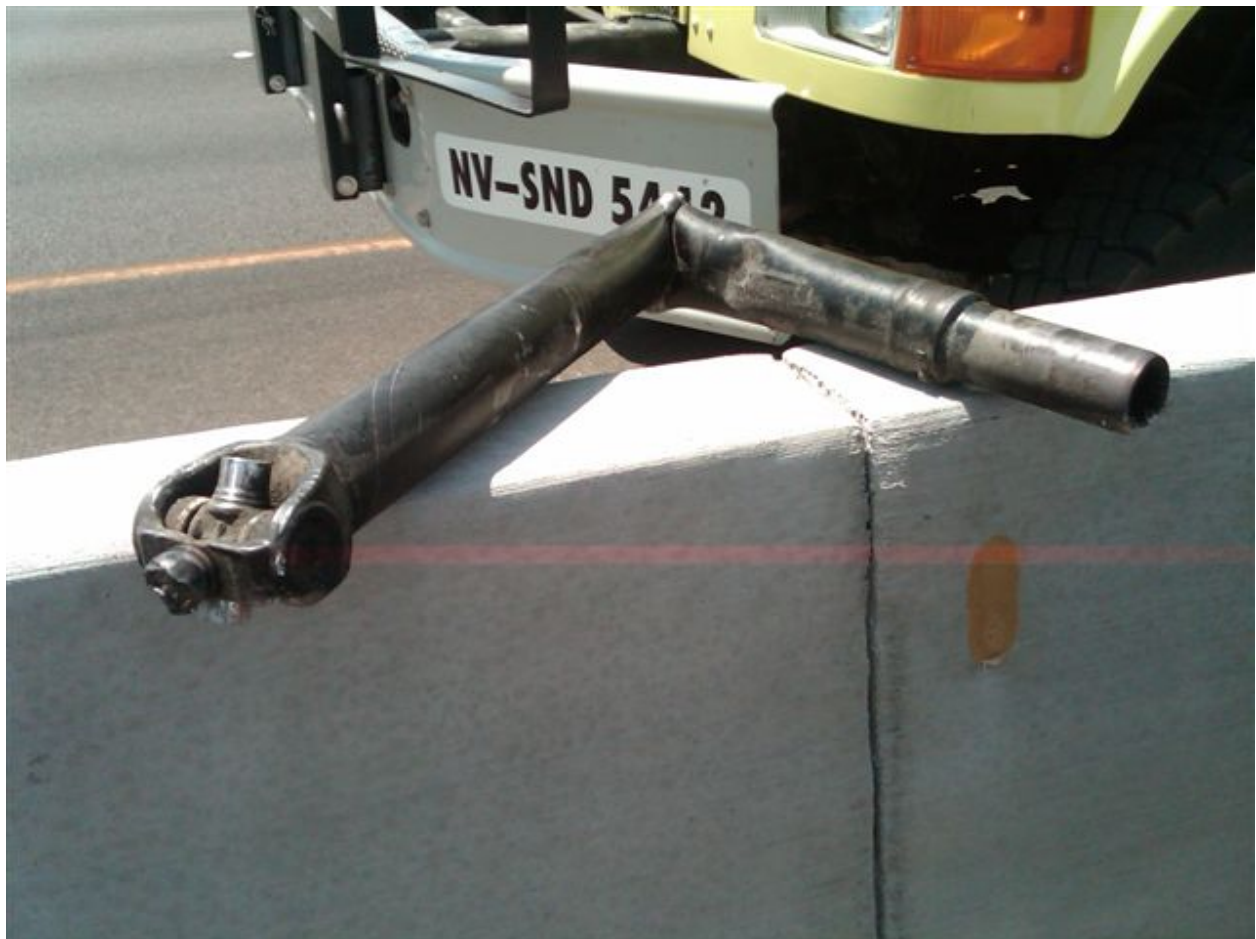
Figure 2 Driveshaft recovered at scene
