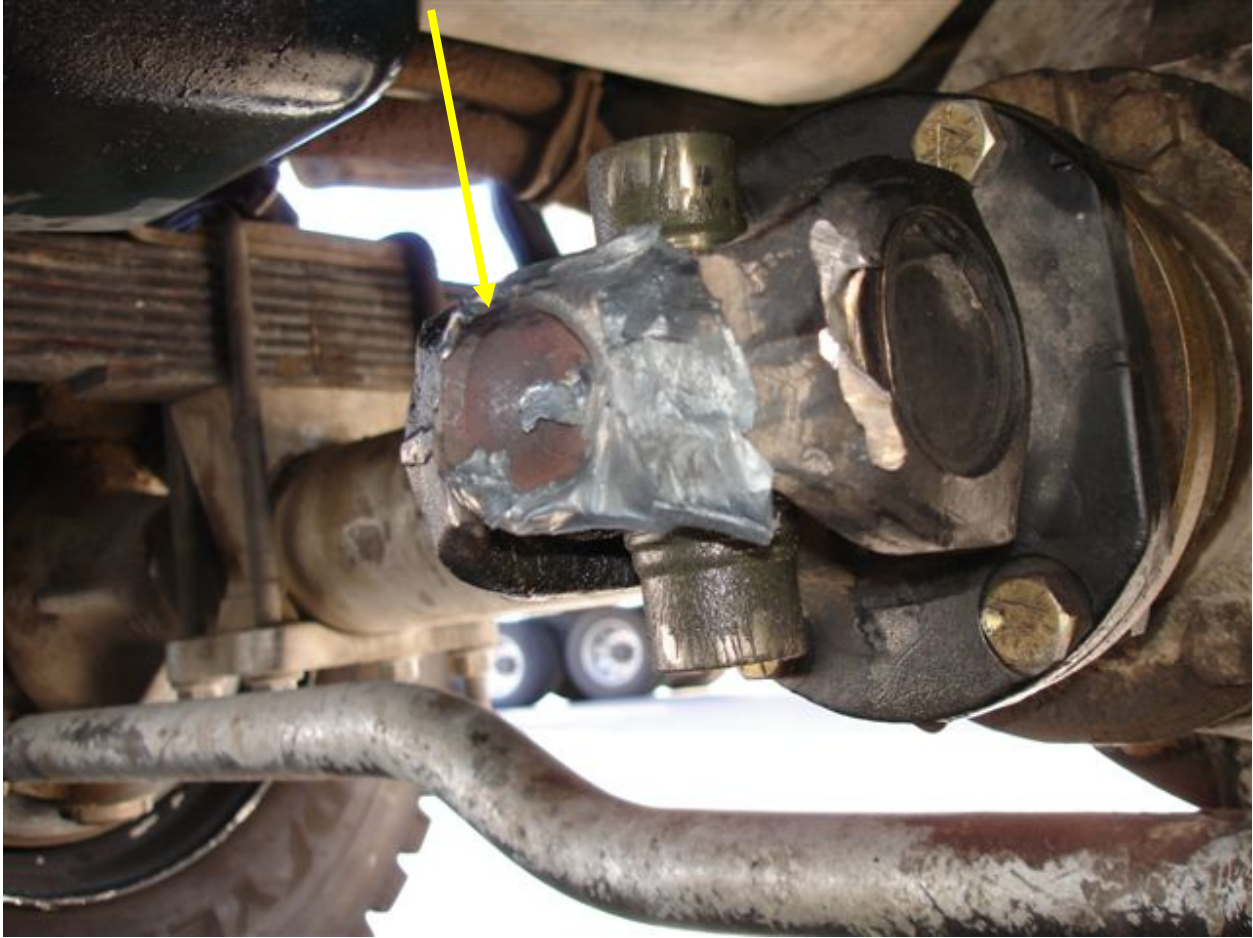
Figure 3 Front Axle Yoke (Note rust color and signs of lack of grease in the seat)
