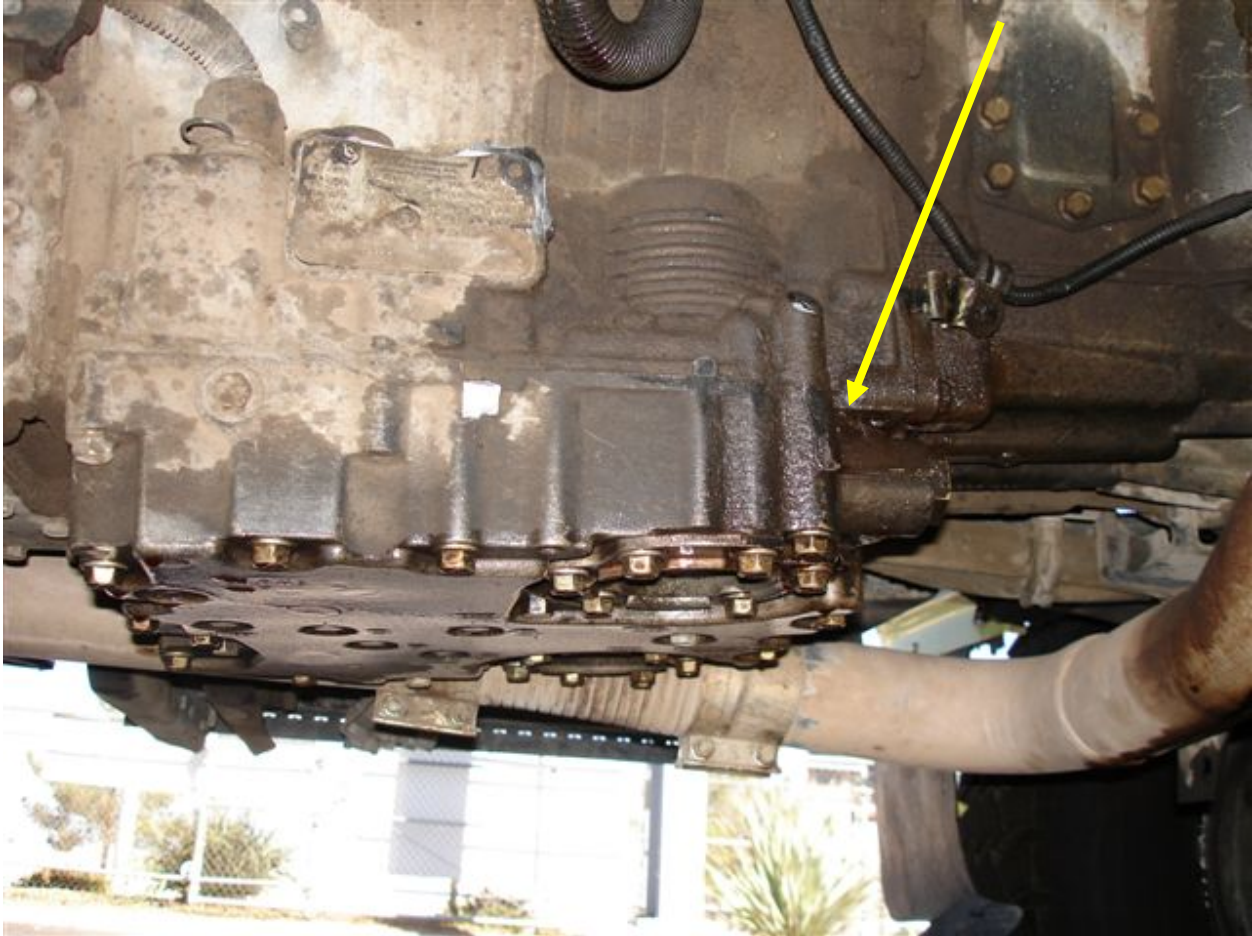
figure 6 Transmission Cracked and Leaking from driveline hitting the case of the transmission.
