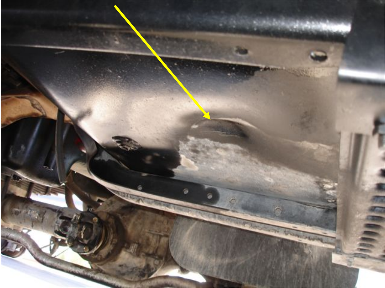
Figure 5 Fuel tank dented and leaking.
