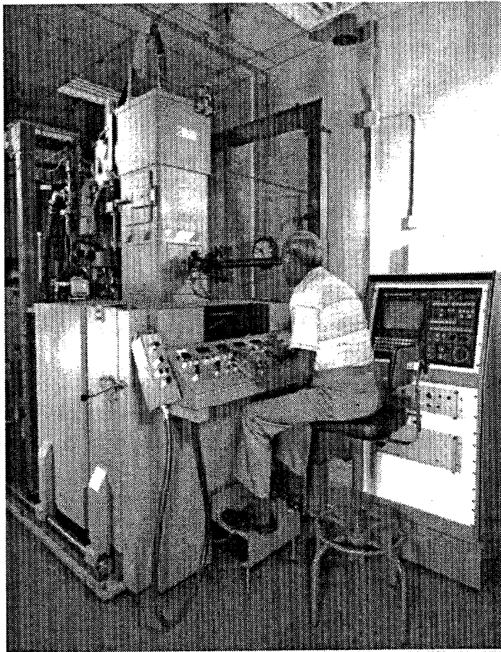
Fig. 17. Leybold-Heraeus Electron Beam Welder, shown here with J. D. Hudson, can make precision microwelds and high depth-to-width ratio deep penetration welds in a range of materials.
