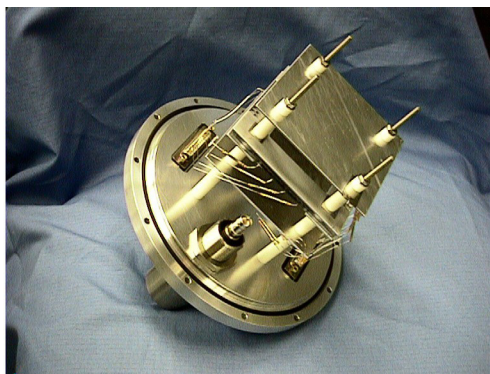
Fig. 1. Photograph of neutron detector developed for this project (a Neutron Micromegas detector using ^3\text{He} as the converter and process gas).
