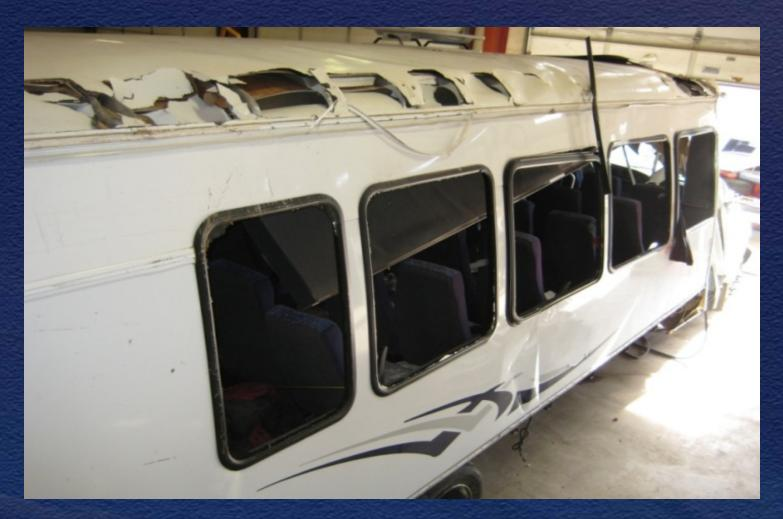
• roof crush minimal; 15 passengers ejected
