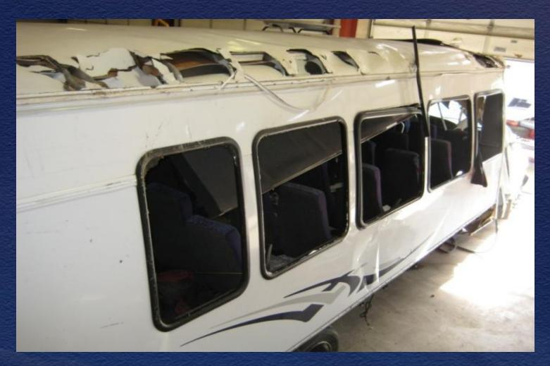
roof crush minimal; 15 passengers ejected
