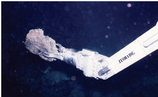
A piece of pillow lava is collected by a mechanical arm of a Remotely Operated Vehicle (ROV) from great water depths on the submerged southern slope of Kīlauea Volcano. To collect the sample of choice, the mechanical arm is precisely manipulated by scientists aboard the ROV's mother ship on the ocean surface. (USGS photograph by Peter W. Lipman.)
