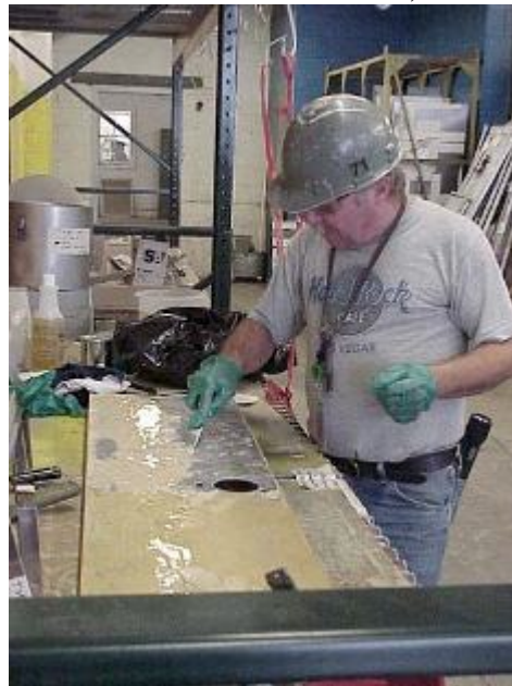
Picture (right): Bruce Trent uses biobased paint stripper at the Portsmouth Naval Shipyard to restore the U.S. naval submarine fleet.
