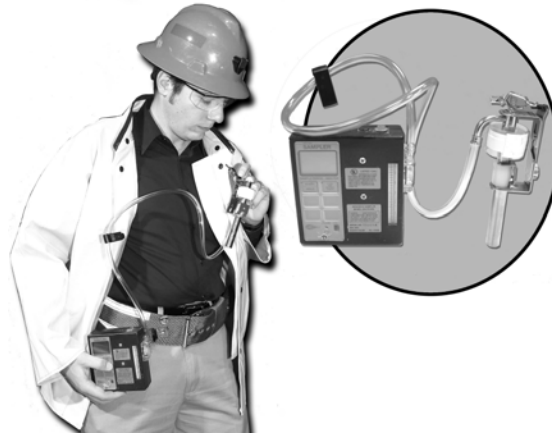
Figure 2-5 Respirable Dust Sampling Setup
