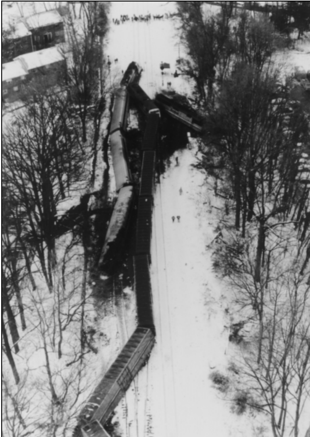
Silver Spring, Maryland. February 16, 1996. The fuel tank of Amtrak's lead locomotive ruptured on impact and the diesel fuel ignited.
