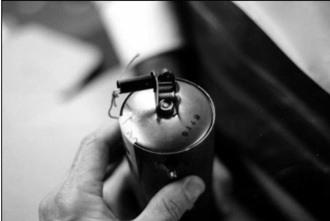
Miami, Florida. ValuJet flight 592. One of the oxygen generators that were improperly carried as cargo.
