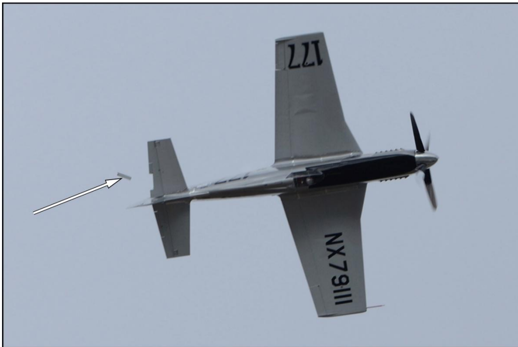
Figure 10. Inboard piece of left elevator trim tab separated.
