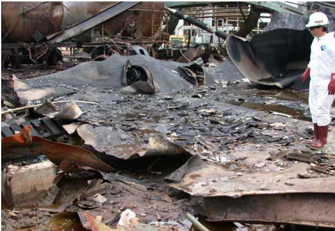
Figure 3. Postaccident photo showing a Safety Board investigator standing on flattened portion of railroad tank car DBCX 9804.
