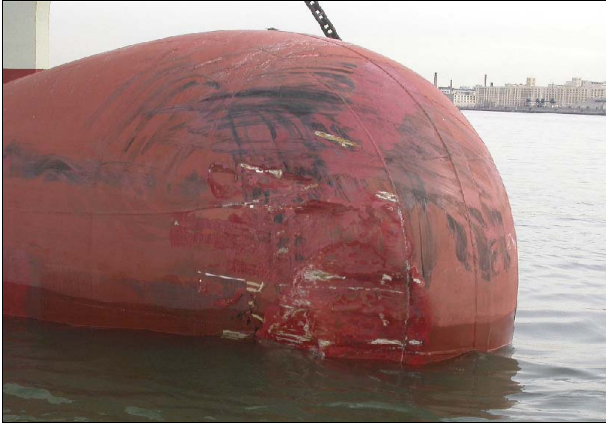
Figure 8. The scraped and dented bulbous bow on the Orange Sun .
