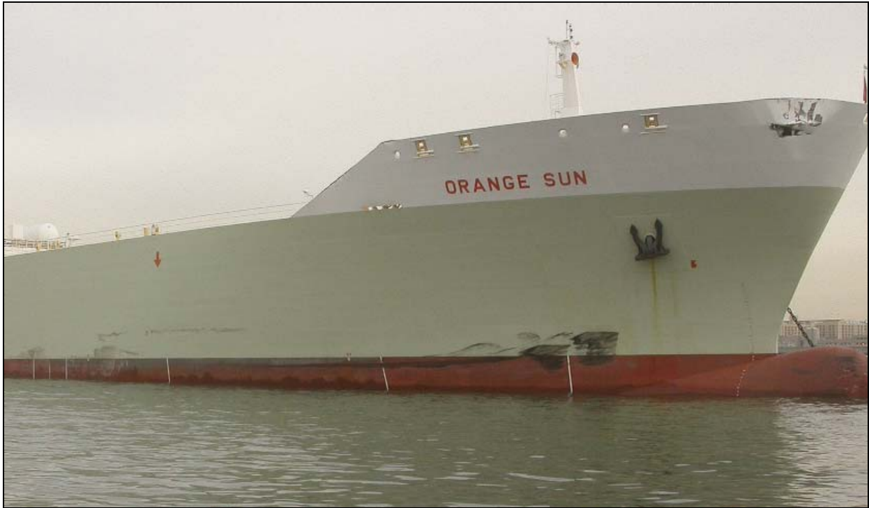
Figure 6. Starboard-side scrapes and smudges on the Orange Sun .
