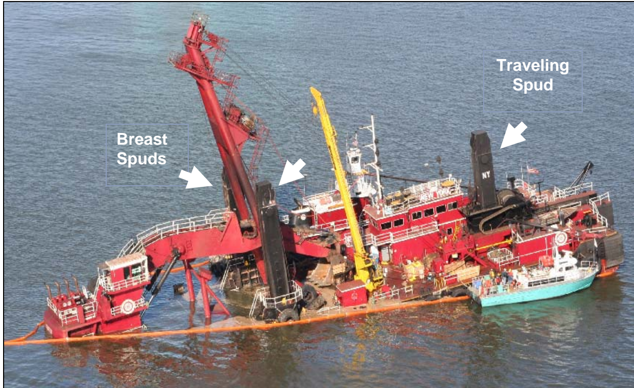
Figure 9. The New York after the allision, with its submerged bow resting on the breast spuds.
