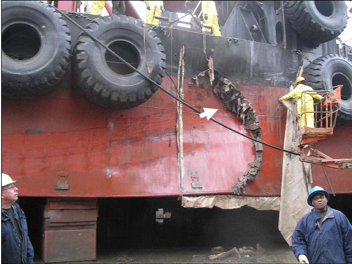
Figure 10. The curved tear in the portside hull of the New York . Photo by Great Lakes Dredge & Dock Company.
