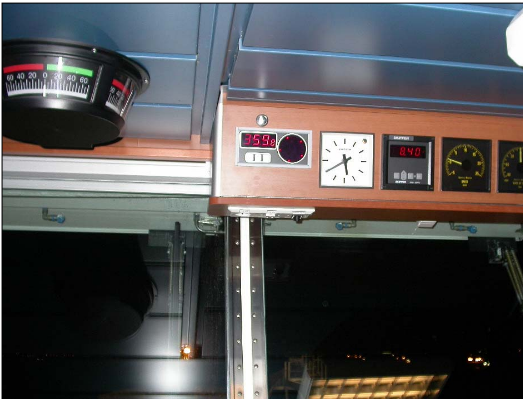
Figure 5. The Orange Sun 's rudder angle indicator, visible in the upper left corner.
