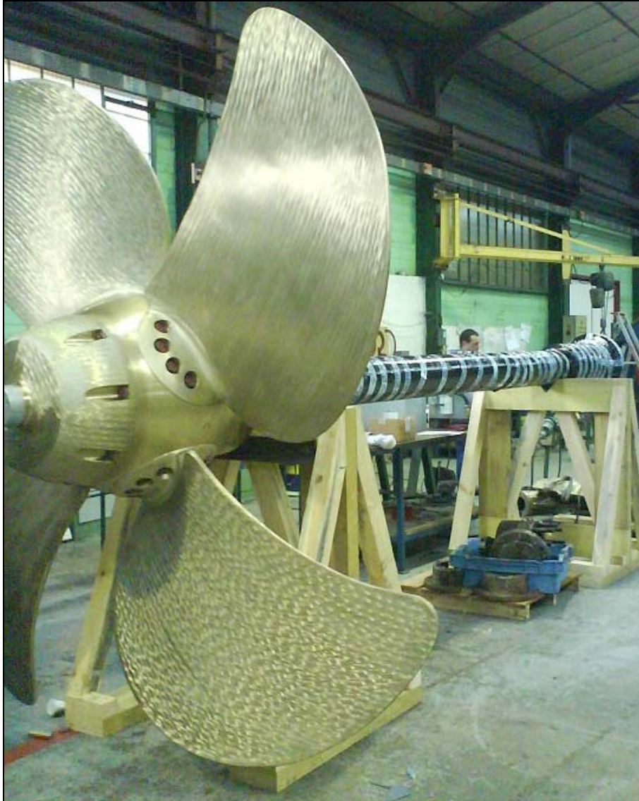
Figure 11. Controllable pitch propeller with adjustable-angle blades and main rotating shaft, similar to the one on the Orange Sun . Photo by Masson Marine.
