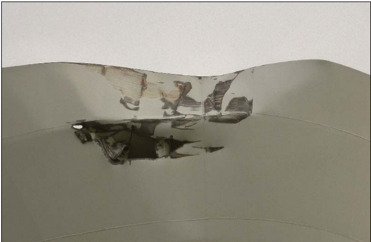
Figure 7. Inset, puncture, and scraping to the Orange Sun 's bulwark on the upper starboard-side bow.
