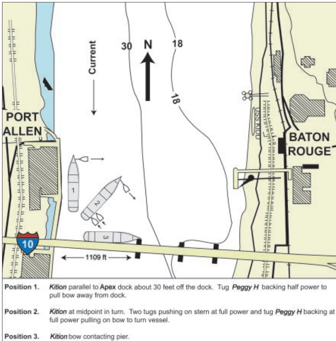
Figure 2. Diagram of Kition moving from the Apex No. 2 dock to its allision with the I-10 bridge pier.
