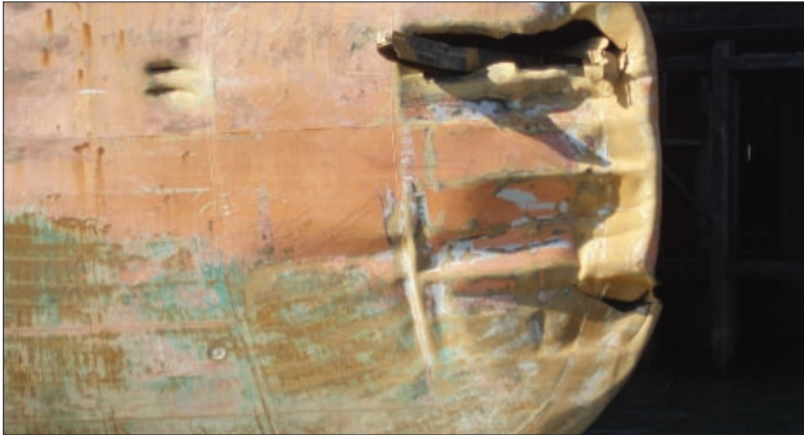
Figure 5. Holed forepeak tank and other damage to the Kition's bulbous bow, shown after the bow was raised out of the water by removing cargo and ballasting the aft tanks.
