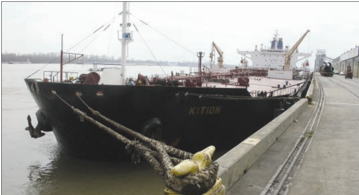
Figure 1. Kition docked downriver of the I-10 bridge after the accident. The vessel's draft (freshwater) on the day of the accident was 44 feet 7 inches.
