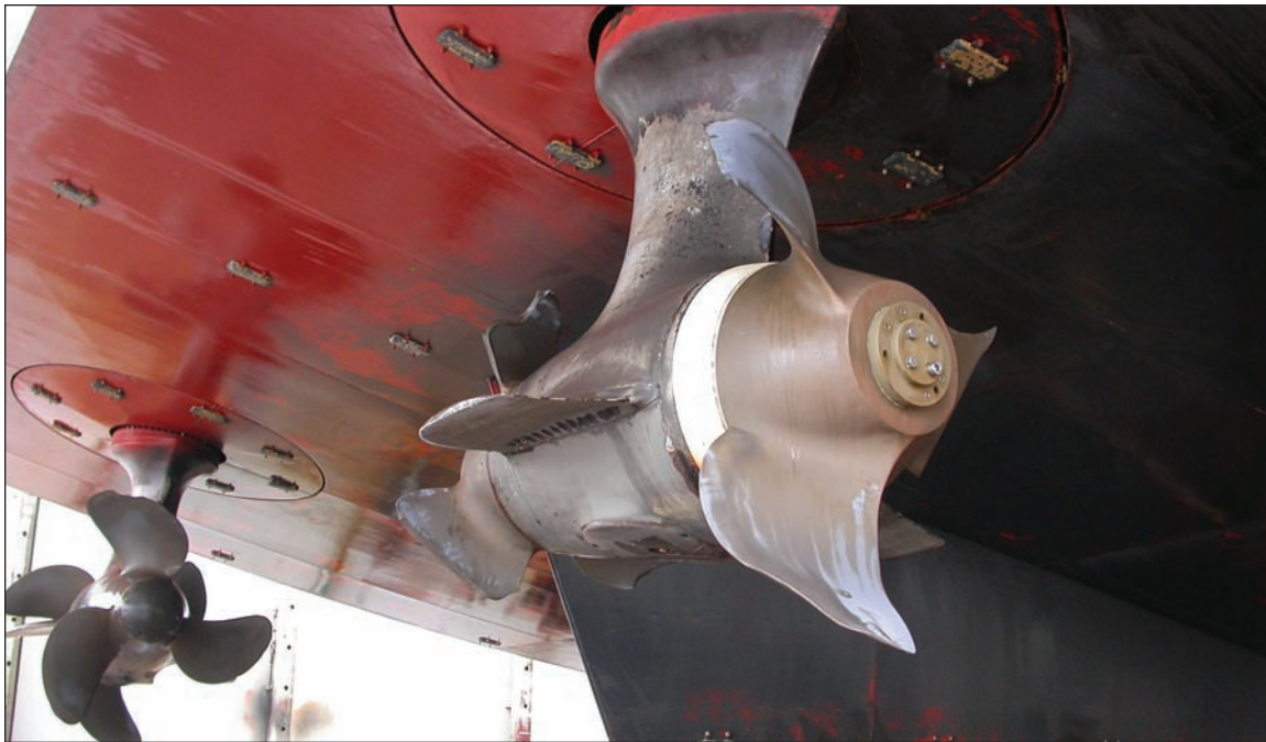
Figure 8. Damage to propeller blades of starboard propulsion thruster (foreground). Port thruster (rear) was not damaged in the grounding.
