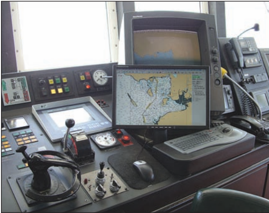
Figure 4a. View of bridge showing location of monitors for Nobeltec (front) and ECDIS (rear) at helmsman's post.
