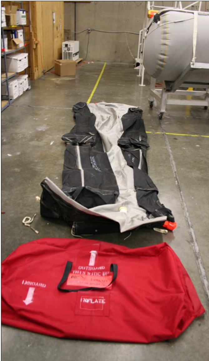
Figure 11. Evacuation slide laid next to a valise in preparation for packing. Photo was taken during tests at the DBC Marine Safety Systems warehouse in November 2007, after the company had labeled its valises THIS SIDE UP (see “Other Actions Since the Accident” section).
