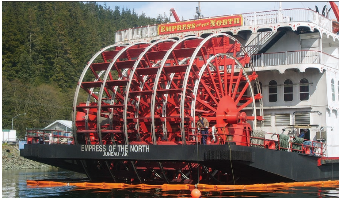
Figure 3. Paddle wheel at the stern of the Empress of the North . To save fuel, the paddle wheel was usually allowed to freewheel during vessel transits, as during the accident voyage, rather than being powered by its driving motor.
