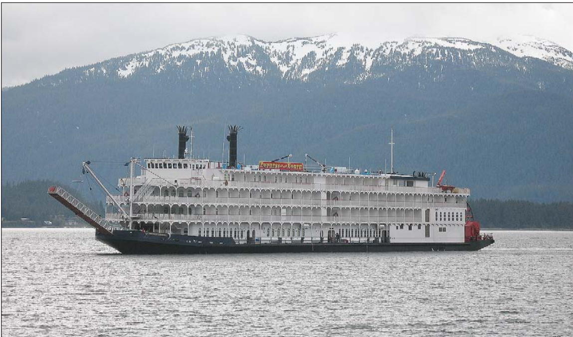
Figure 1. The Empress of the North under way in Auke Bay, Alaska. The newly constructed ship had four passenger decks and was designed to mimic Mississippi River paddle wheelers (the red paddle wheel is barely visible at the vessel's stern). Passengers embarked and disembarked using the gangway at the bow, shown here in the raised position.
