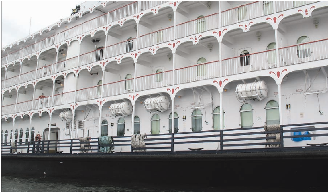
Figure 5. Liferrafts mounted in overhead cradles above the main deck of the Empress of the North .
