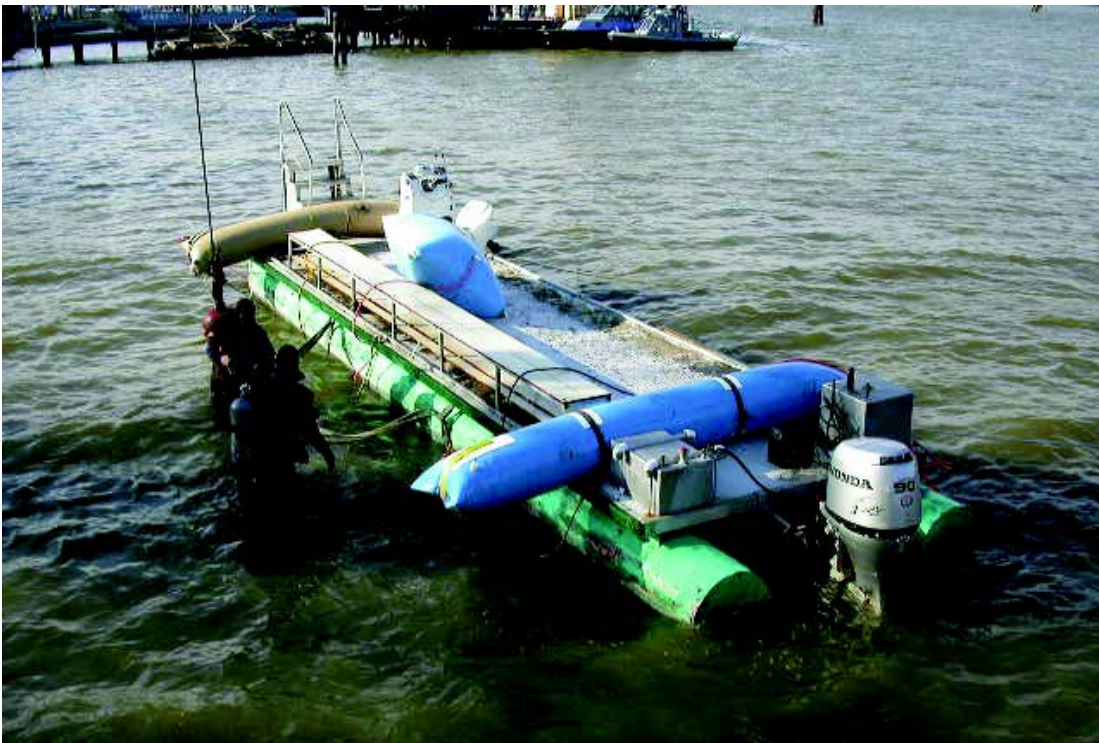
Figure 3. Lady D after being righted the day after the accident. Attached to the deck are airbags that were used to help right the vessel. Most of the deckhouse was missing and never recovered.
