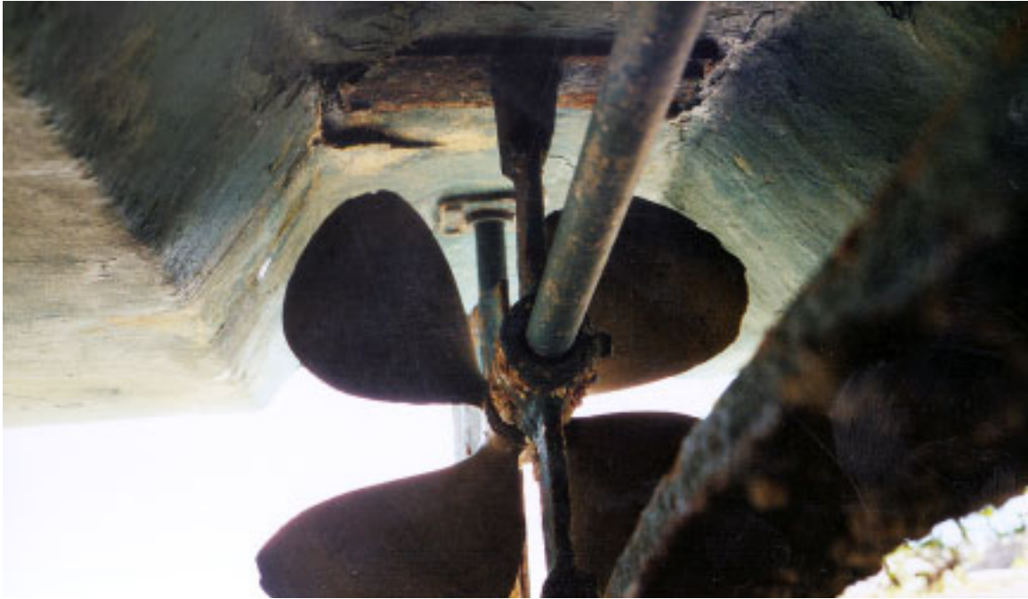
Figure 6a. C-shaped fracture around strut plate.
