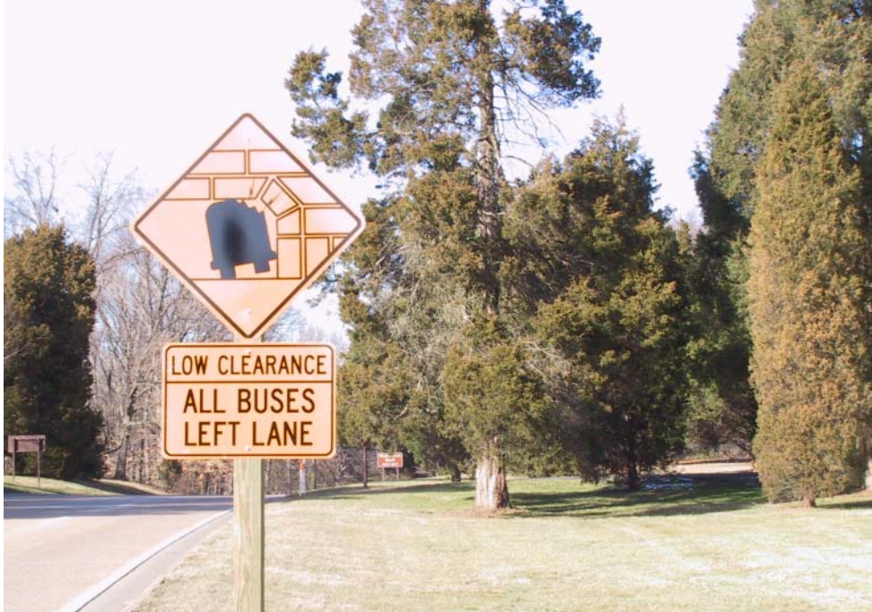
Figure 6. One of the four new warning signs for the Alexandria Avenue bridge overpass.
