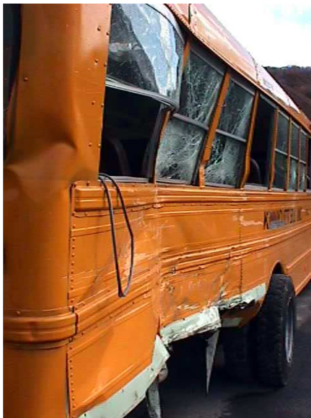
Figure 1. Exterior crush damage of school bus.
