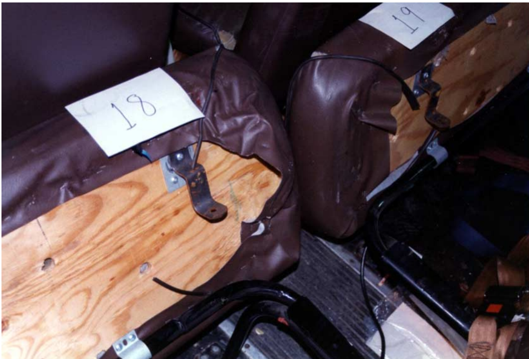
Figure 7. Postaccident view of the bottom of the seat cushions and latching clips.
