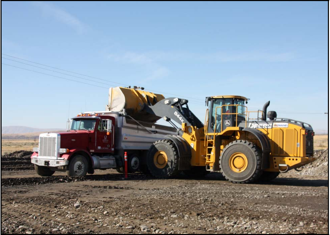
Washington Closure Hanford is using truck and pups to transport waste material to the Environmental Restoration Disposal Facility. (Photo 6)
