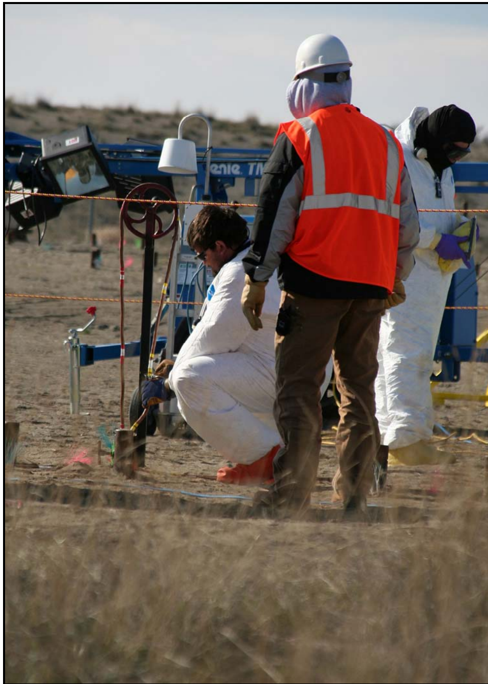
A multi-detector probe used to measure radiation source is retrieved from a cone penetrometer at the 618-10 Burial Ground.
