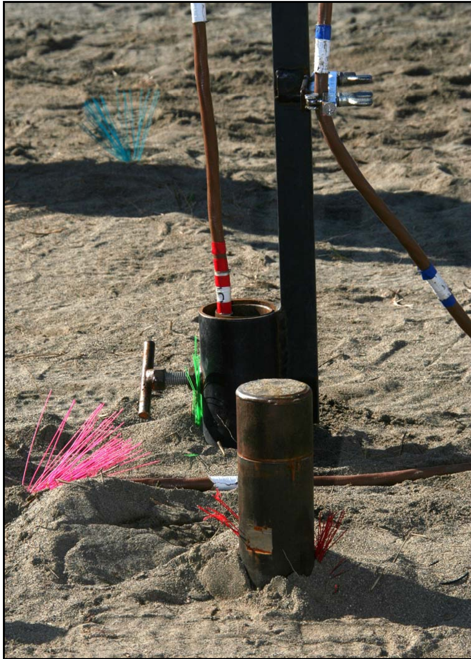
A multi-detector probe is shown at the 618-10 Burial Ground. Measurements are taken each foot with a 3-minute count time. A radiological control technician then checks for contamination as the probe is removed from the cone penetrometer.
