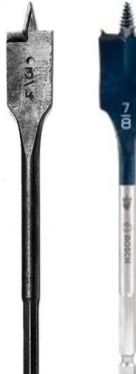
Left: Spade bit Right: Spade bit with spurs
