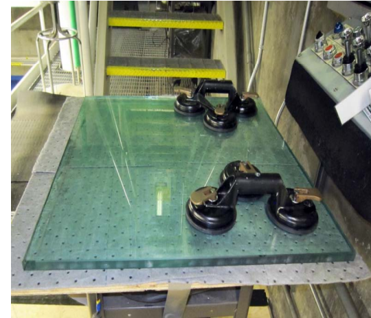
Refurbished hot cell window at 242-A Evaporator
