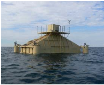
Oscillating water column device: Oceanlinx.
