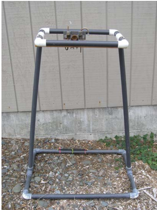
Figure 5 PVC photo framer for photographing permanent 50 x 75 cm plots. A camera (not shown here) is mounted to the top brackets to ensure accurate replicate size. Three corners of the framer's base are aligned with three stainless steel bolts that are permanently fixed in the rock. One of the three bolts is notched with the plot number, and indicates the orientation of the plot.
