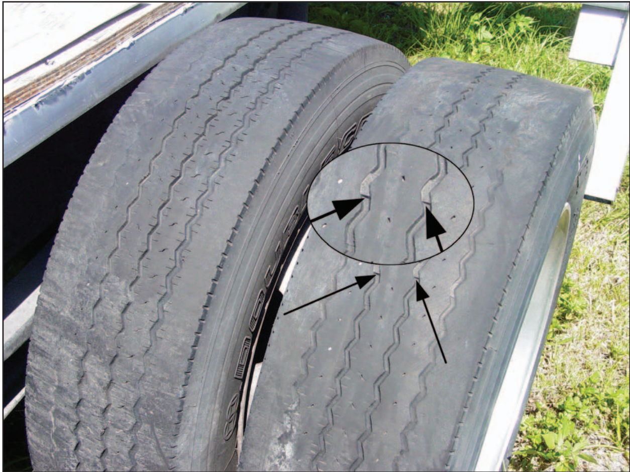
Photo 1. Illustrates the significant wear on one set of the rear tires. Arrows indicate the visible wear bars.
