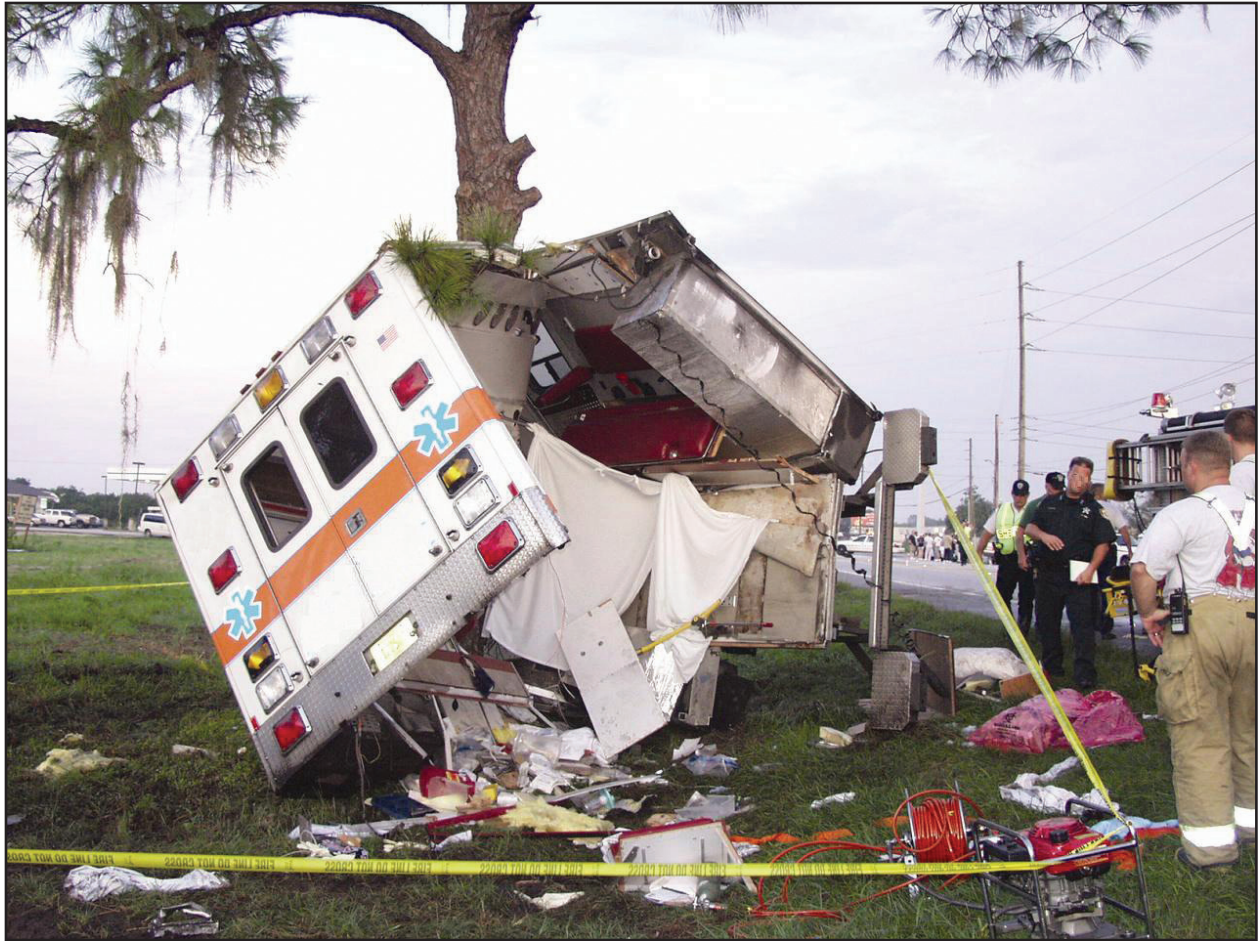
Photo 3. Patient compartment of ambulance after crash, showing the separation of curbside wall and roof. (Photo courtesy of the County Sheriff's office)
