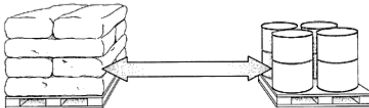
FIGURE 12 - Aisle space to allow free air flow and access between rows of stacked pesticides
