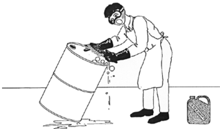
FIGURE 23 - Decontamination of a pesticide container - the inside and outside are being cleaned with detergent and water - highly contaminated rinsings should be saved for disposal with other major toxic waste
