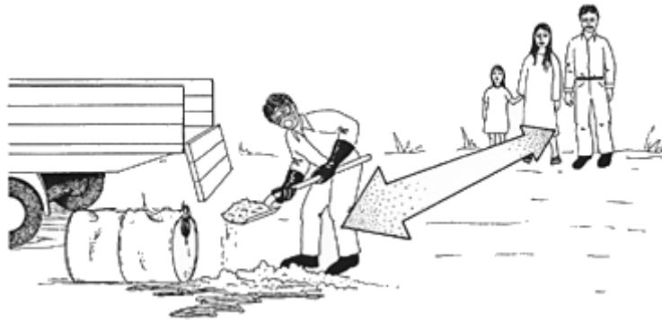
FIGURE 19 - Spill, caused by a pesticide drum falling off a vehicle, being covered by soil - people are kept away from the spill
