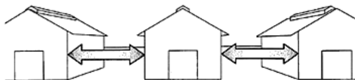
FIGURE 4 - The pesticide store should have three sides free to allow access to fire-fighting equipment in an emergency
