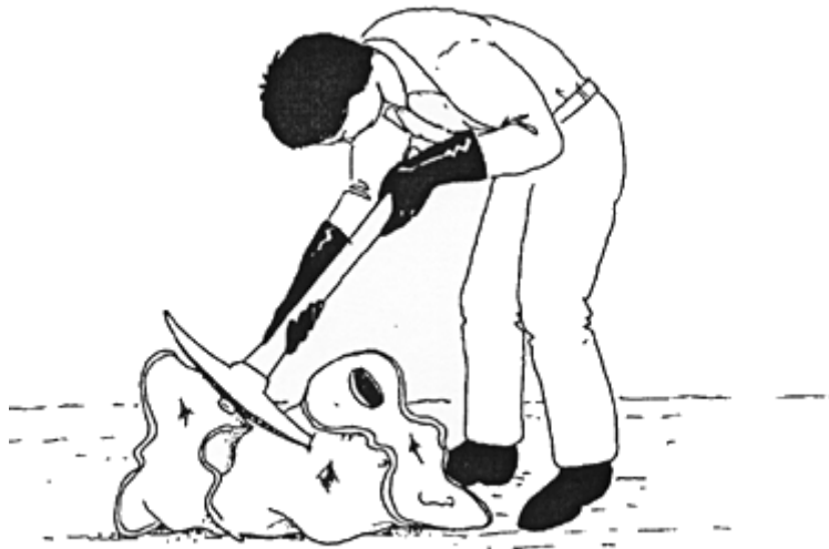
FIGURE 25 - Metal container being crushed so that it cannot be reused - it will be collected for central disposal by the national authority
