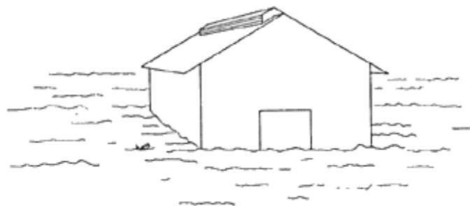
FIGURE 3 - The pesticide store should not be sited in an area subject to flooding, especially during seasonal rains
