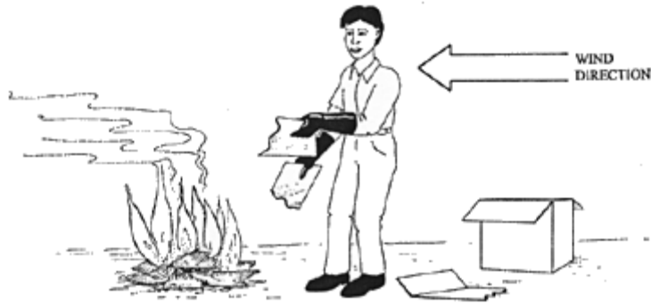
FIGURE 24 - Disposal of lightly contaminated cardboard pesticide container on a fire, ensuring that fumes travel away from personnel
