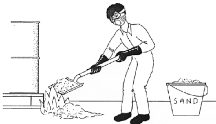
FIGURE 28 - Extinguishing a small fire in a pesticide store using shovelfuls of sand or earth from a container
