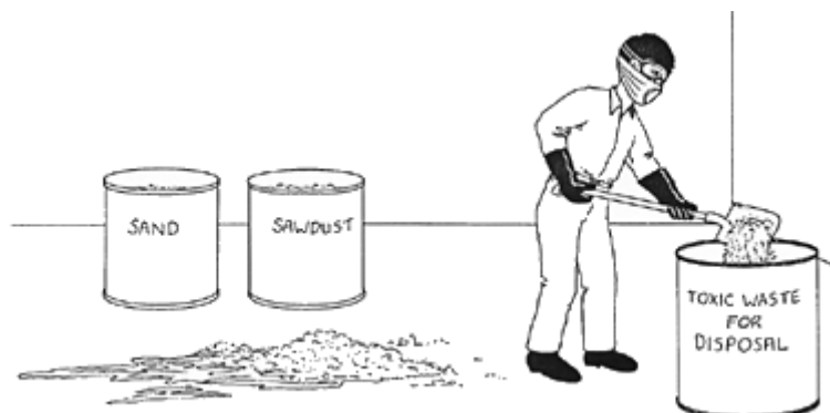
FIGURE 21 - Spill soaked up by sand or sawdust being carefully swept up by the storekeeper and placed in a container to be collected and taken for central disposal by the national authority
