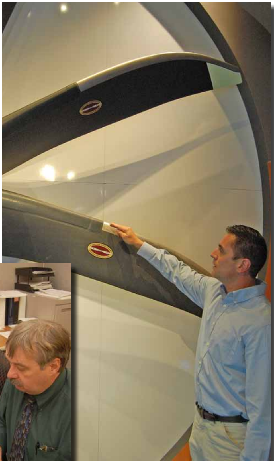
Above: Steven Nogas, a Defense Contract Management Agency quality assurance lead in Windsor Locks, Conn., points to a heated blade on a NP2000 propeller. (Photo by Patrick Tremblay, DCMA Public Affairs)
