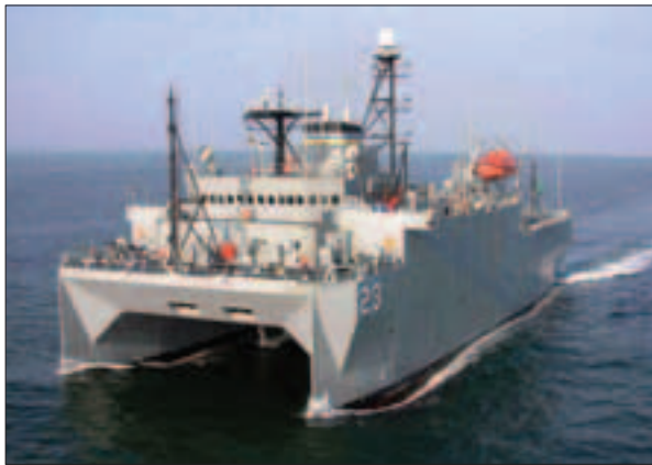
The Military Sealift Command's ocean surveillance ship Impeccable (T-AGOS 23) supports the Navy by using both passive and active sonar arrays to detect and track undersea threats.
