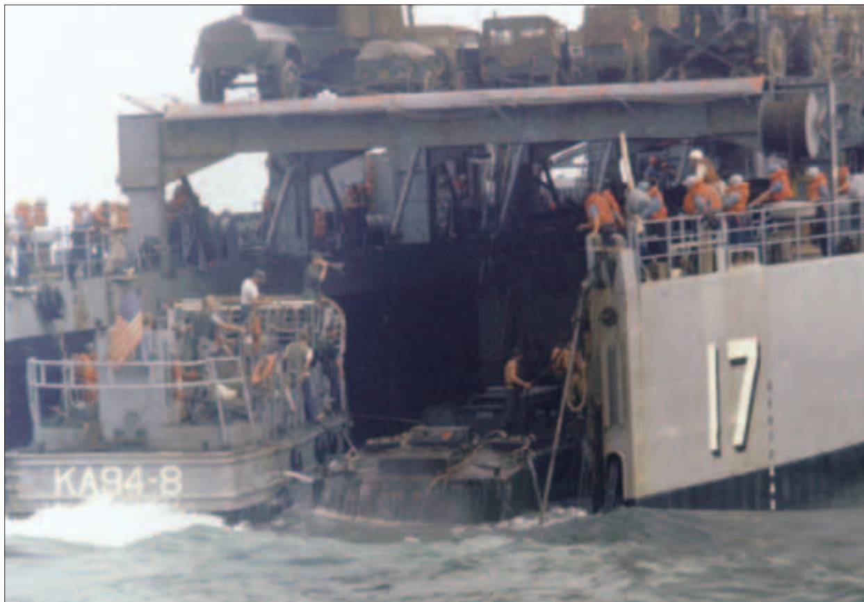
A landing craft and a tracked landing vehicle enter the well deck of dock landing ship Catamount (LSD 17).
