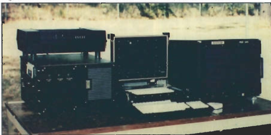
Part of the setup for the Small Tactical Terminal, a direct-readout, two-person transportable weather satellite data receipt and analysis system.
