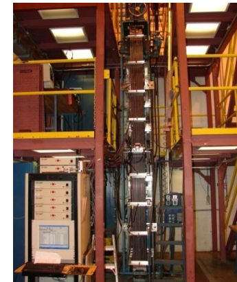
Mechanical Assembly Test Forced Vibration & Seismic/LOCA
