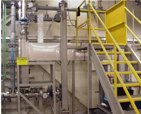
VISTA Loop 5x5 testing pressure drop & vibration
