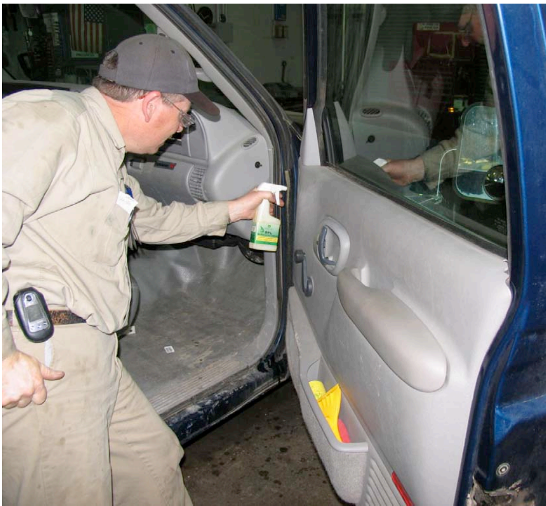
Mechanic Steve Bolden uses biobased penetrating oil to lubricate ORNL vehicles so they run smoothly.
