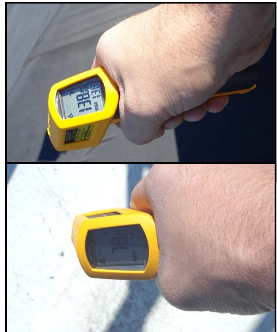
(Top) Roof temperature prior to biobased roof coating. (Bottom) Roof temperature after the biobased roof coating was installed.
