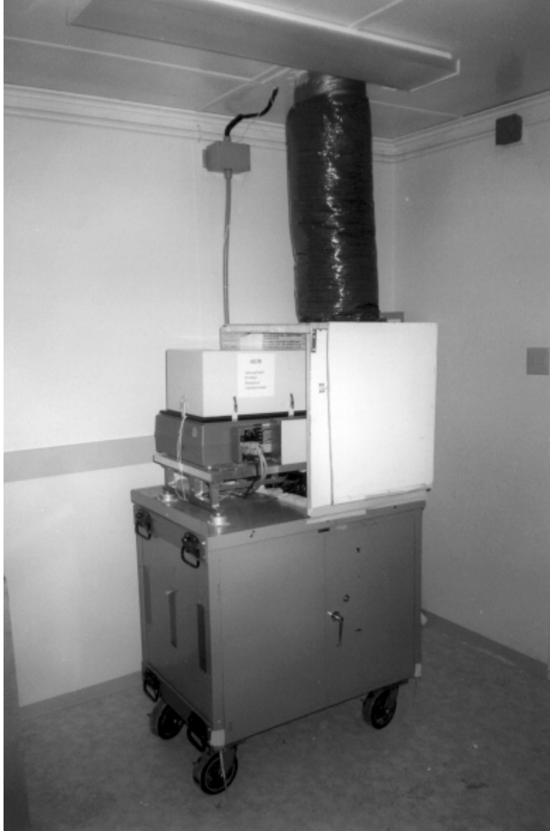
Figure 1.1. The AERI prototype as it was configured inside the SGP CART CF optical trailer near Billings, Oklahoma. The white box and the black chimney-like structure acts to insulate the AERI scene mirror and blackbodies from the ambient room air while providing a vertical view of the sky through a ceiling hatch. The edge of the viewing hole in the white box was responsible for the obstruction in the sky FOV.
