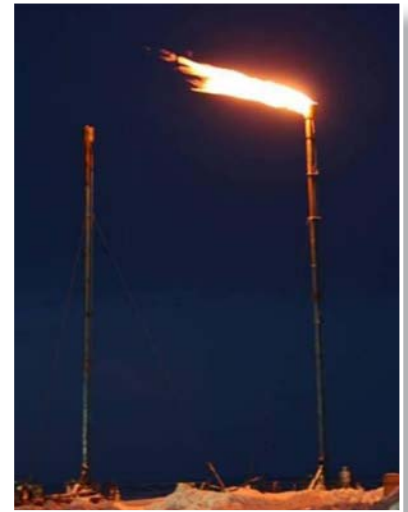
Natural gas flare at Mallik site during 2008 well test using depressurization technique. (Courtesy of Natural Resources Canada and Japan Oil, Gas, and Metals National Corporation)
