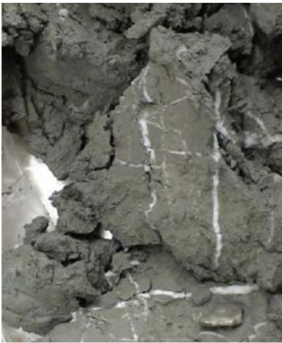
Hydrate-filled fractures found in marine sediment. (Courtesy of the UBGH-01 [Korea] Science Party)
