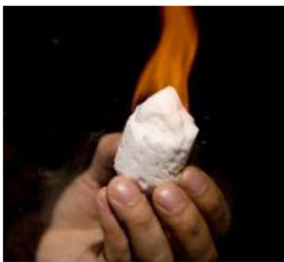
Methane hydrate dissociating with the methane ignited – "burning ice." (Courtesy of National Research Council Canada)
