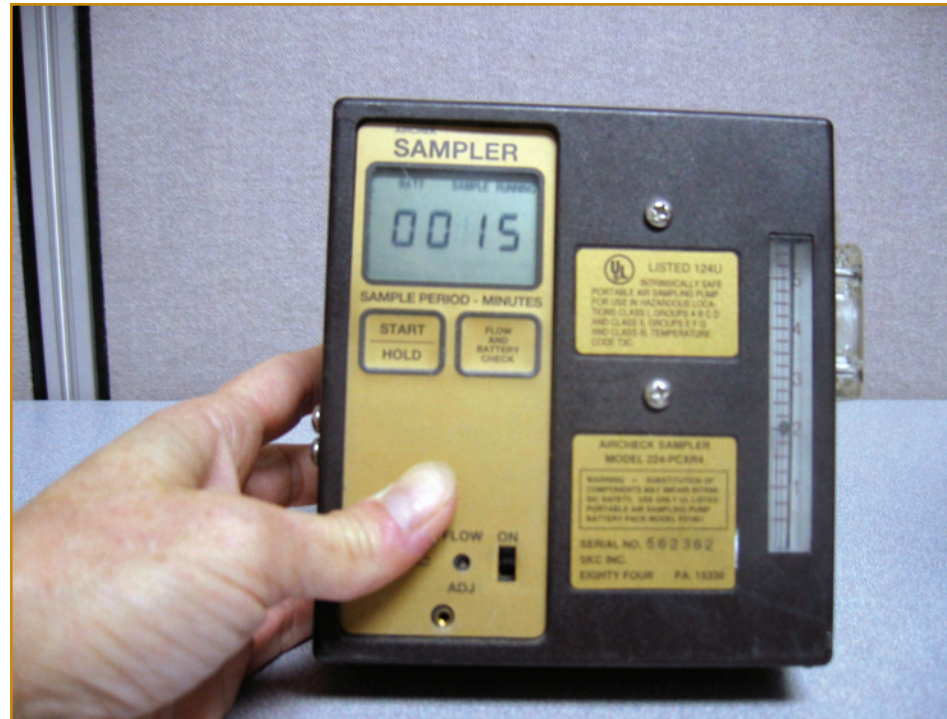
Figure 1: Select a personal air sampling pump that provides a suitable range of air flow rates. The pump shown here requires a special added low-flow valve to adjust the air flow rate to the correct level for sampling EtO, which is 100 milliliters of air per minute (ml/min) or the equivalent of 0.100 liters per minute (l/min).
