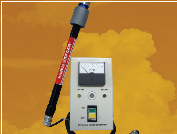
Portable EtO gas-detection meters are available to check for leaks around equipment such as sterilizers, tanks, fittings and pipes that contain EtO. Leak testing is generally performed using hand-held EtO detection meters (a type of portable direct-reading instrument). See the related Section 3.A.iii - Emergency Alert Provision .
