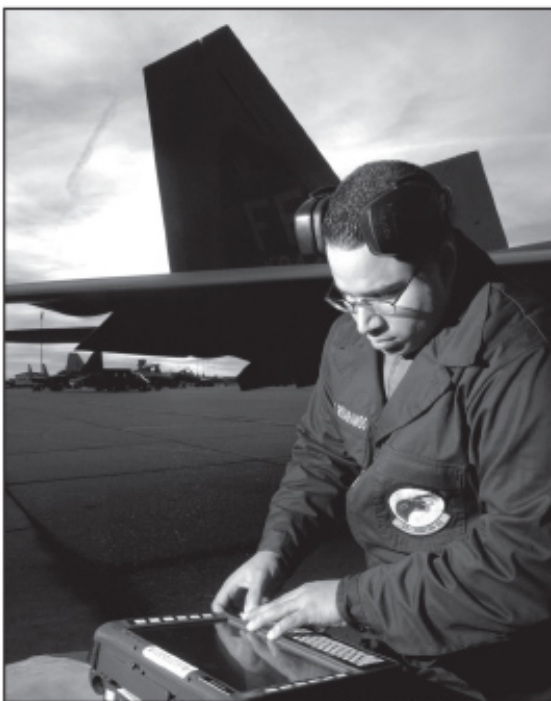
Photo by Tech. Sgt. Ben Bloker Staff Sgt. Ramon Rosaromos checks the weapons load status on a portable maintenance adapter in preparation for the F-22A Raptor's first real-world Operation Noble Eagle mission. Sergeant Rosaromos is a weapons loader from the 27th Aircraft Maintenance Squadron.
