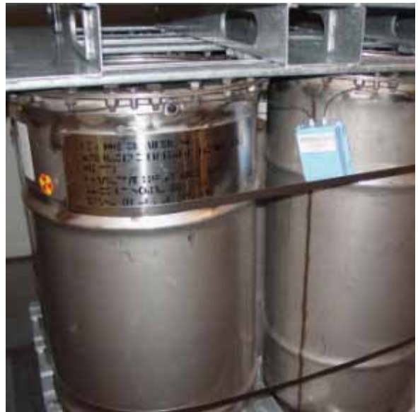
Sandia optical seal in place on drums of radioactive materials.
