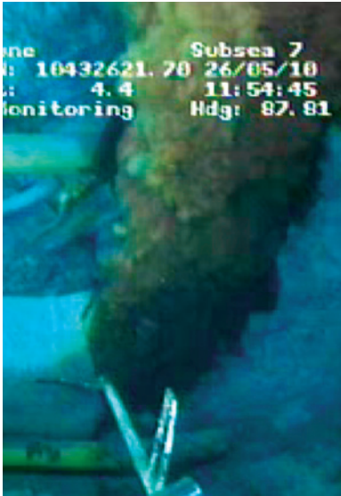
Oil spews unchecked from the Deepwater Horizon's severed riser in this video frame taken May 26. When the rig sank, the riser broke off, settling on the sea floor.
