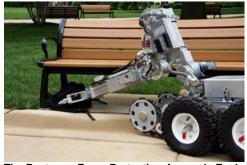
The Pentagon Force Protection Agency's Explosive Ordnance Disposal (EOD) Unit uses one of its robots to move a simulated suspicious package during a presentation today in the Pentagon Center Coutyard. PFPA's EOD team is one of the assets the agency has to respond to reported suspicious packages. PFPA launched a public awareness campaign today, aimed at encouraging Pentagon employees, visitors, and commuters to report suspicious activity: "If You See Something, Say SomethingTM."
