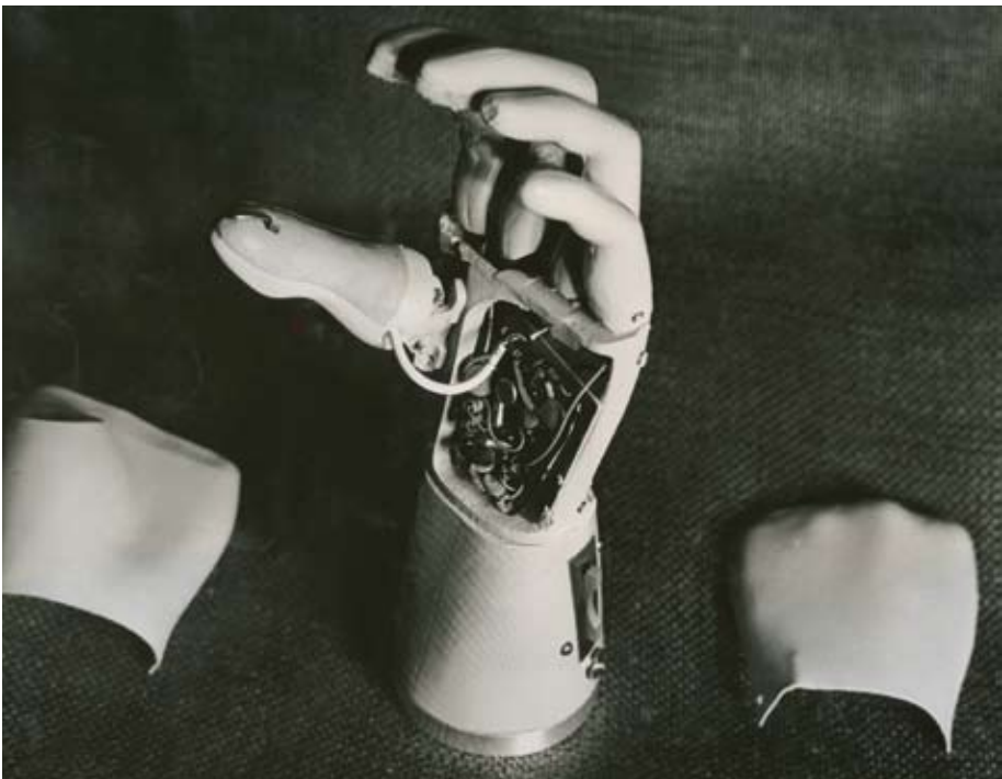
USAMBRL developed an electromechanical artificial hand that provided an amputee with a controlled, secure grasp. (U.S. Army, 1968).
