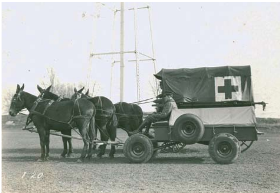
Mule-drawn, rubber-tired ambulance being tested and compared to an iron-rimmed, spoke-wheel ambulance, 1930. (Carlisle Barracks Collection, photo by USAMHI).
