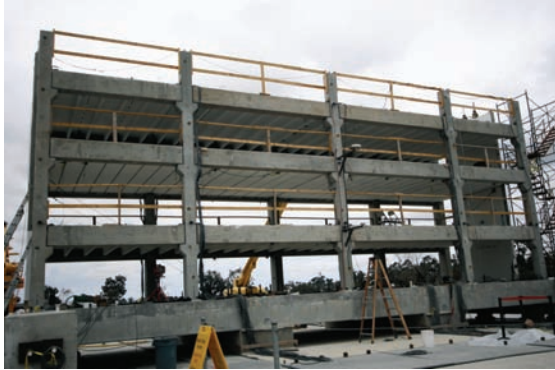
Figure 2. Test of a half-scale model of a three-story parking garage on the shake table at the University of California, San Diego, Englekirk Structural Engineering Center. The UCSD shake table is an element of the NEES infrastructure, the largest shake table in the United States, and the only outdoor shake table in the world. This study is supported by NSF, NEESinc, the Precast/Prestressed Concrete Institute, and the Charles Pankow Foundation. ©2008 by UCSD Jacobs School of Engineering.
