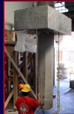
Tests on pile-deck connections at UW
