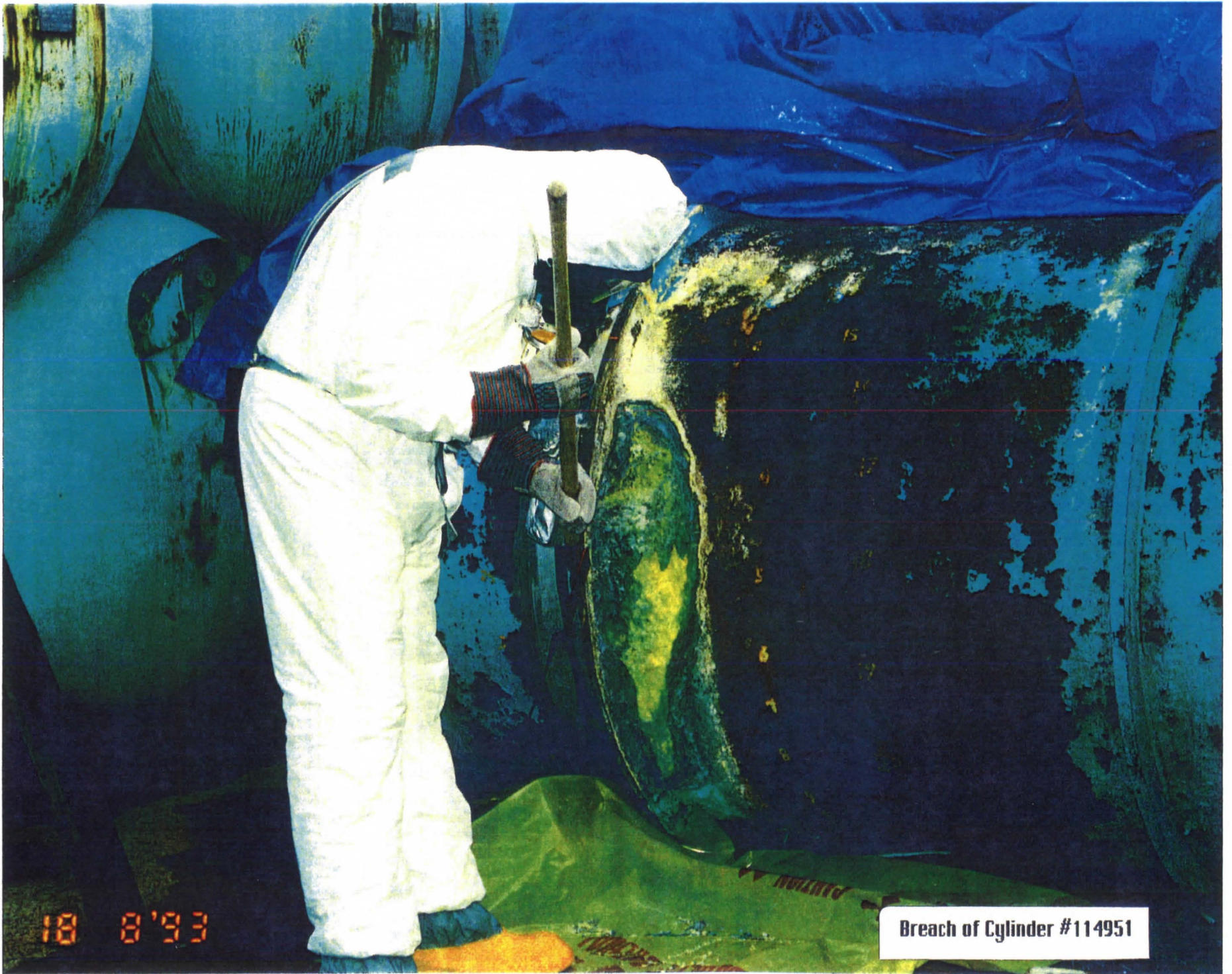
Figure 2 Breached Cylinder at Oak Ridge K-25 Site
