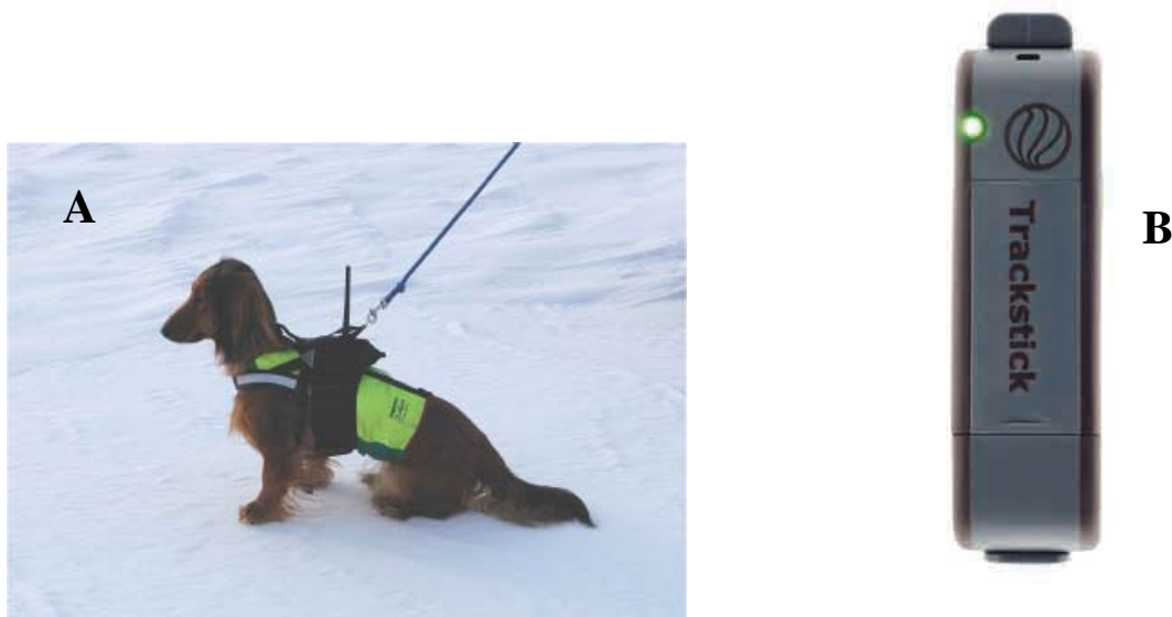
Figure 3.8: A: Tara with the Garmin 220 system. Both the GPS receiver and the UVF transmitter are built into one compact unit. The positions are sent in real-time to a Garmin 220 hand-held map plotter. The UVF antenna is shown in picture B: The Trackstick unit with a built-in GPS receiver and memory stick for data logging.
