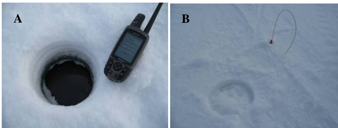
Figure 3.5: Small training oil spills used for the field training. A: 400 ml of weathered Troll crude ( 200^{\circ}\text{C}+ ) in a 30cm hole in the first year ice. B: The hole is covered with snow and ice chips and marked with a small white cord.
